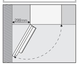
Check that there is a gap of at least 11 3/4" (299 mm) between the wall (or similar) and the coffee machine so that you can open the door wide enough to remove the left-hand bean container (minimum door opening angle of 120°).
