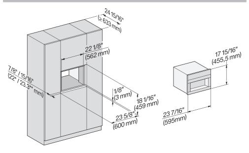
Combination with other Miele Built-in Appliances is possible. If the coffee machine is to be built in above another appliance, there must be a full-width, closed shelf between them. If the machine is to be combined with a suitable built-in dishware/ food-warming drawer, no shelf is required in between.
